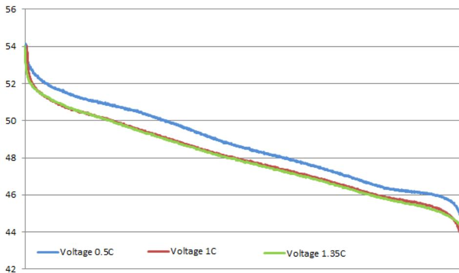
Graph 5: Sirius 7.1kW.h Voltage at multiple discharge rates
